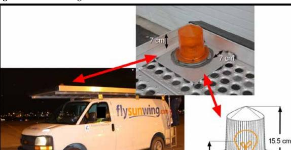
Figure 2. Grote beacon light installation on the maintenance van
