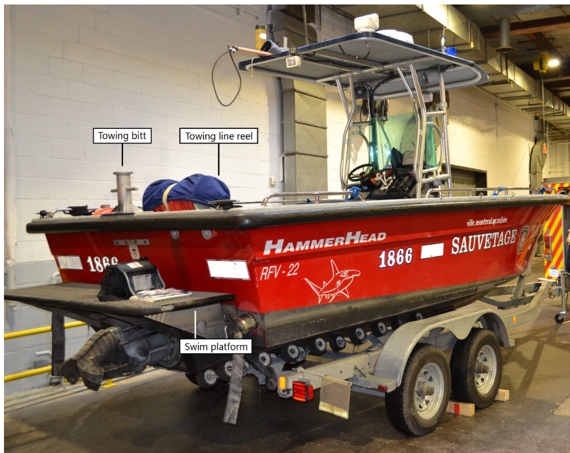
Figure 1. HammerHead RFV-22 (sister boat to the occurrence boat) with tow cable reel, towing bitt and swim platform labelled (Source: TSB)
