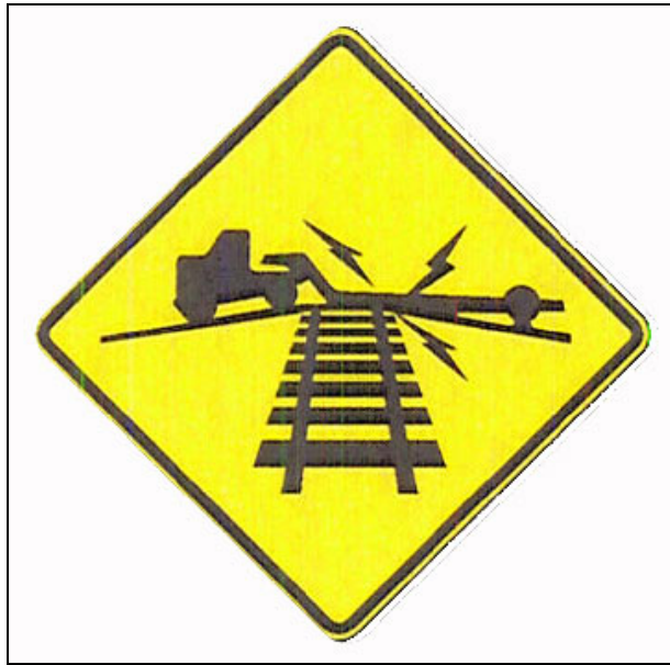
Figure 4. United States Department of Transportation standardized low ground clearance W10-5 sign
