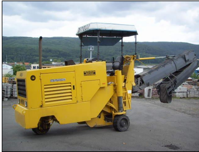
Photo 1. Cold-planer of type being transported on lowboy trailer
