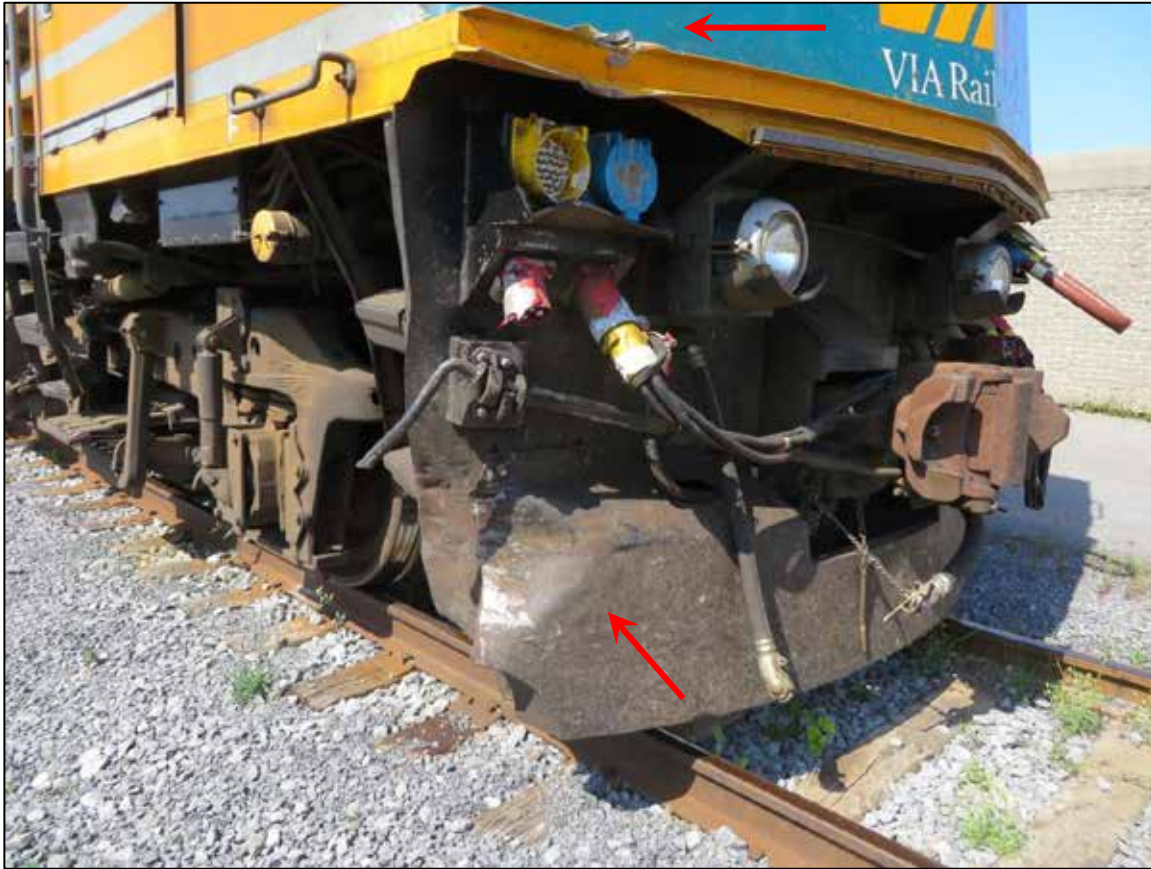
Photo 1. Locomotive VIA 6424 showing impact damage (red arrows)
