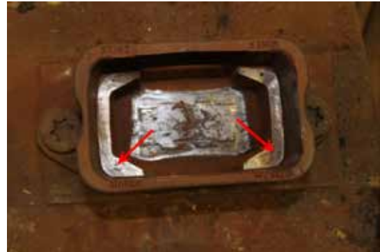
Photo 6. Left side constant contact side bearing cage. Arrows point to worn areas where the metal portion of the CCSB has made contact with the cage
