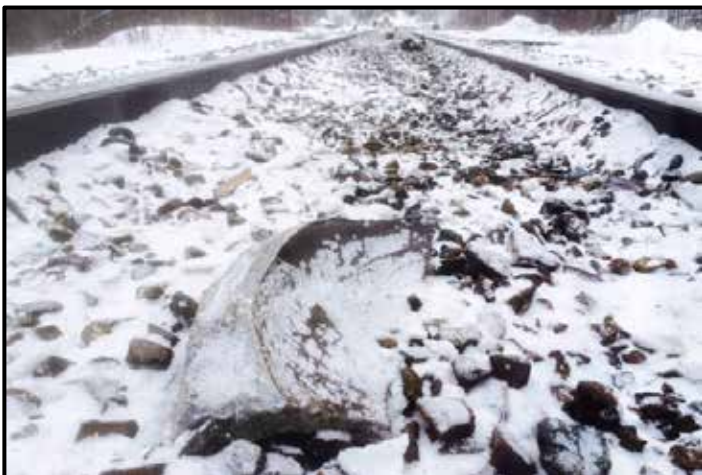
Photo 6. Tread section with plate located at Mile 20.55 (Source: Canadian National Railway Company)
