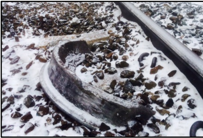
Photo 7. Tread section with plate located at Mile 21.00 (Source: Canadian National Railway Company)
