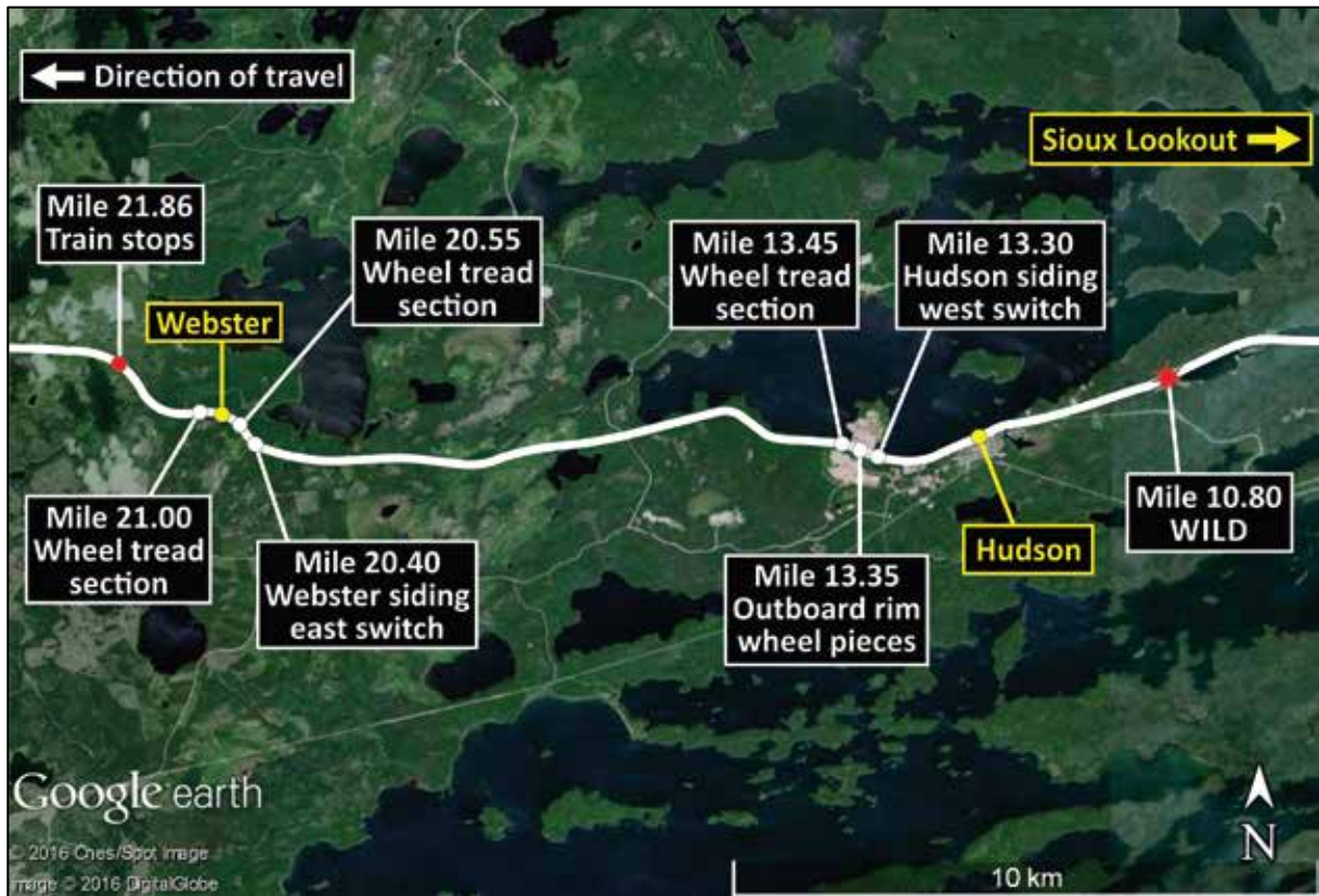
Figure 2. Site diagram between the Hudson wheel impact load detector site (Mile 10.80) and where the train came to a stop (Mile 21.86) (Source: Google Earth, with TSB annotations)
