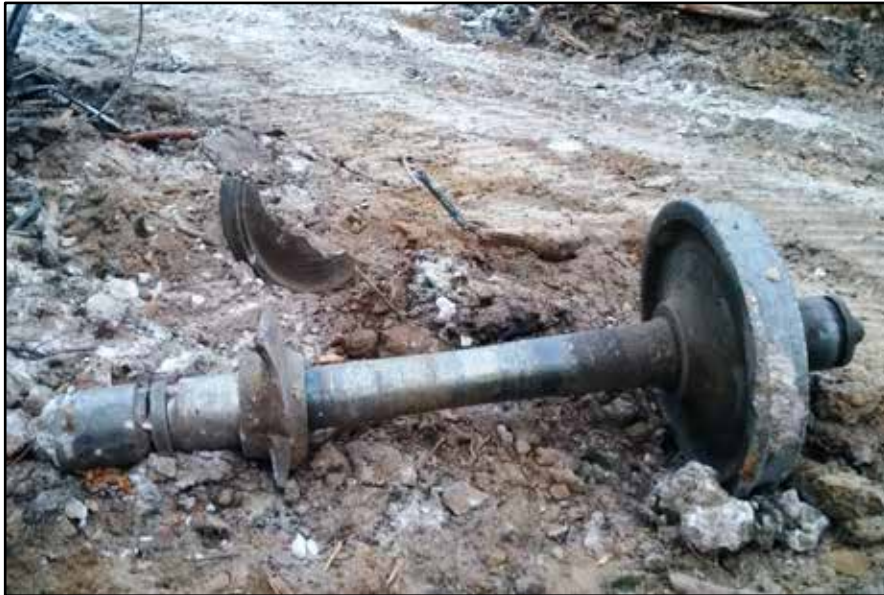
Photo 2. Wheel set with failed L1 wheel (Source: Canadian National Railway Company)
