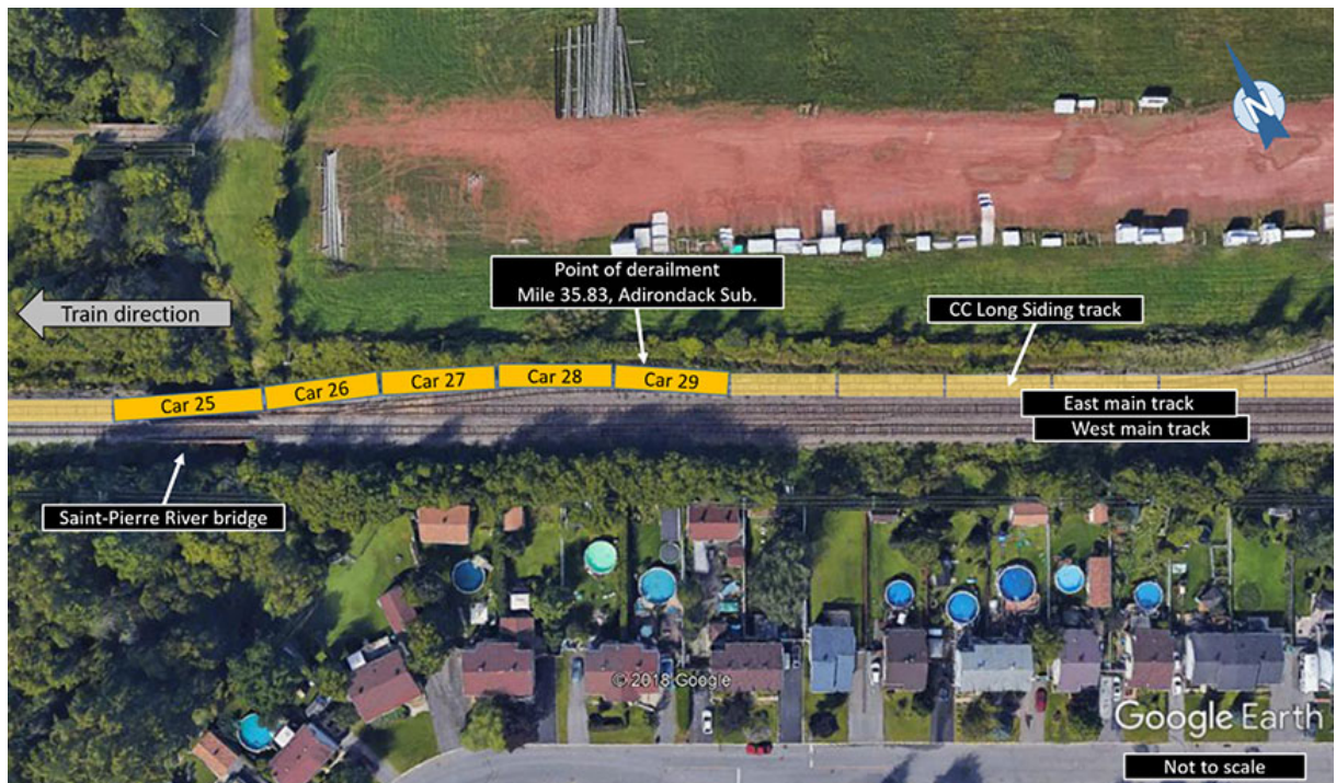
Figure 2. Derailed cars at the north end of the CC Long Siding track at Delson, Quebec (Source: Google Earth, with TSB annotations)
