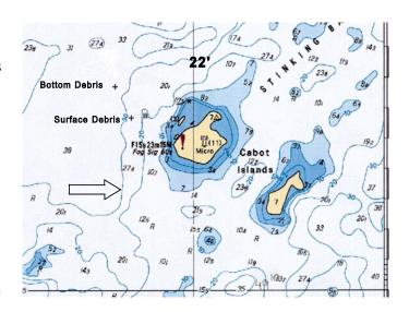
northeast. The distribution of wreckage items was consistent with the tidal current. Less-dense components, such as the main rotor, panels, and the tail boom, were deposited to the southwest (see Appendix A). The wreckage was approximately 600 feet farther out from, and in line with, the estimated location of the floating netload of barrels observed immediately after the accident.
