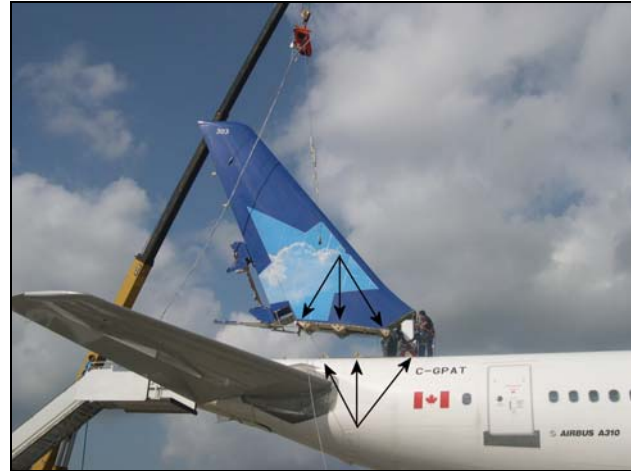
Photo 2. Removal of the VTP and a view of the position of the main attachment fittings
