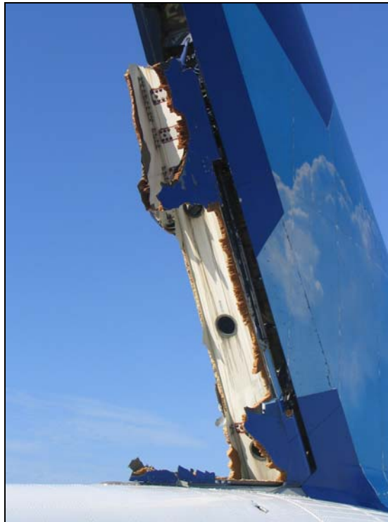
Photo 1. Right-side view of vertical tail plane and rudder residuals
