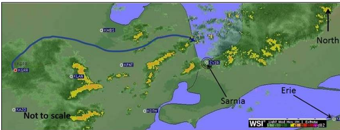
Figure 2. Dispatcher's view of the aircraft's flight track at approximately 1915, showing the actual flight path (blue line) and weather. The weather depiction was generated by a base reflectivity radar source, using the lowest of the reflectivity angles. (Source: ExpressJet, with TSB annotations)
