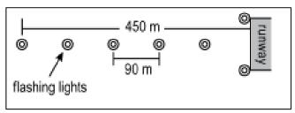
The ODALS was serviceable at the time of the occurrence, and was turned on automatically when the pilot activated the ARCAL.
