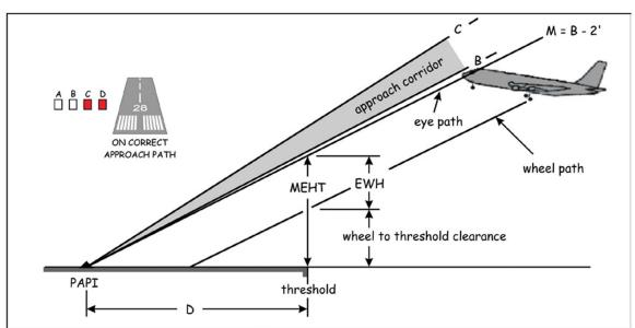
Figure 5. Precision approach path indicator: pilot eye path to wheel path (Source: Transport Canada, Transport Canada Aeronautical Information Manual, AGA – Aerodromes [12 October 2017], section 7.6.4.3)
