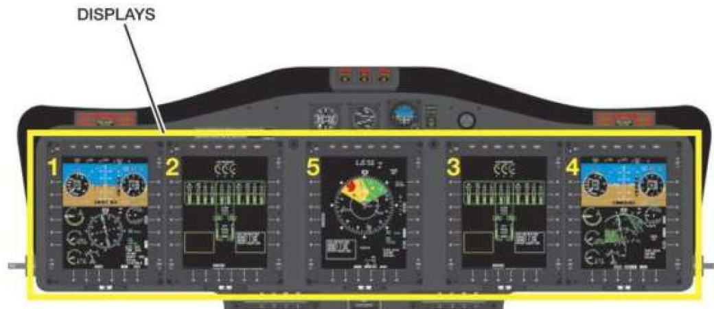
Figure 6. Canadian Helicopters Offshore S-92A instrument panel - standard configuration (Source: Canadian Helicopters Offshore, Sikorsky S-92A Standard Operating Procedures for 704 Commuter and 702 Aerial Work , Issue 4.0 (01 May 2019), Section 1.14.2)
