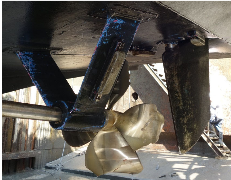
Figure 3. Damage to port propeller and rudder (Source: TSB)
