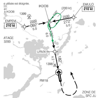
Figure 16. Diagram showing the flight path as the aircraft was exiting the holding pattern at IKDOB (Source: NAV CANADA, Canada Air Pilot [CAP], CAP 6: Quebec [effective 05 October 2023], with TSB annotations)
