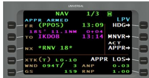
Figure 9. Main navigation page en route to IKDOB before the holding pattern was programmed (Source: Universal Avionics, FMS Trainer v4.1.0.600)
