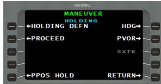
Figure 13. Main navigation page after activating the PROCEED [proceed to] function to exit the holding pattern (Source: Universal Avionics, FMS Trainer v4.1.0.600)
