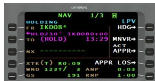
Figure 11. Main navigation page when the aircraft was established in the holding pattern at IKDOB (Source: Universal Avionics, FMS Trainer v4.1.0.600)
