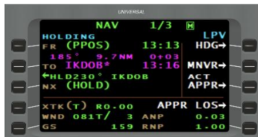
Figure 10. Main navigation page en route to IKDOB after the holding pattern was programmed (Source: Universal Avionics, FMS Trainer v4.1.0.600)
