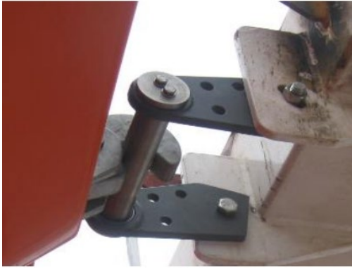
Figure 7. A free-fall lifeboat release hook in position (Source: Viking-Norsafe AS)
