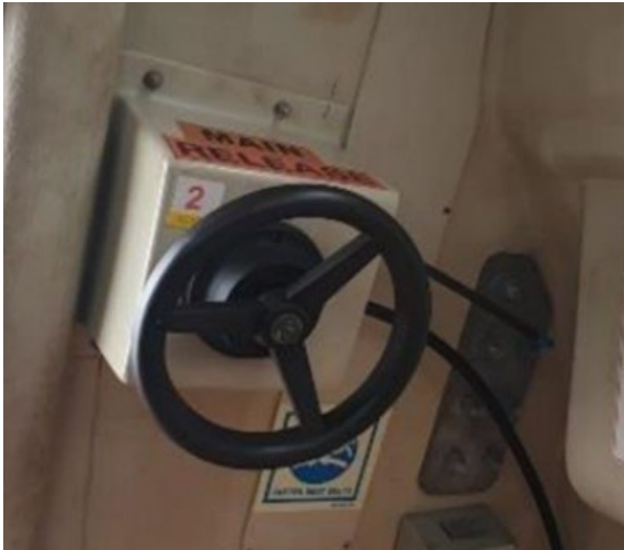
Figure 12. The release wheel on the lifeboat (Source: Columbia Shipmanagement Ltd.)
