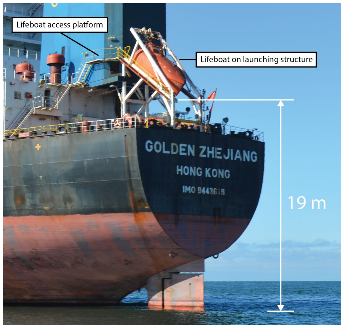
Figure 2. The free-fall lifeboat stowed on the launching structure and the lifeboat access platform (Source: TSB)
