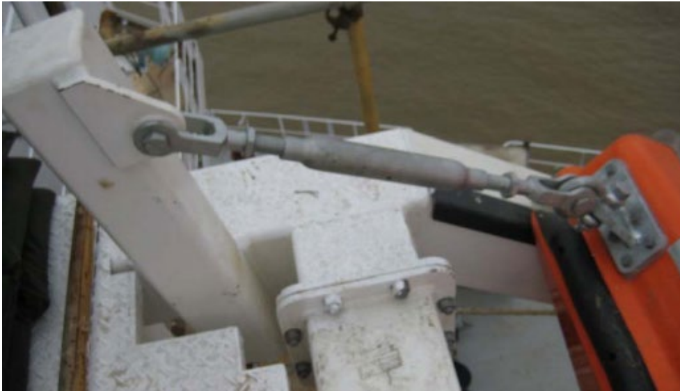
Figure 11: Turnbuckles to secure the lifeboat during training and maintenance, as recommended by the manufacturer (Source: Viking-Norsafe AS)
