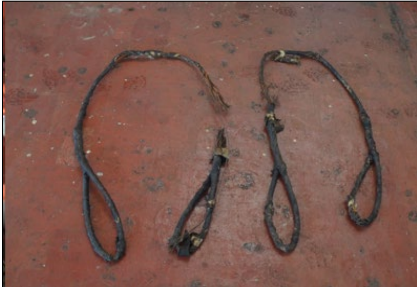
Figure 10. The 2 failed cables, post-occurrence (Source: TSB)
