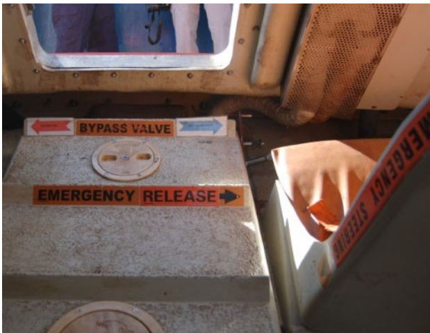
Figure 13. The release station, viewed from within the lifeboat and facing the door, showing labels in place at the time of the occurrence (Source: TSB)
