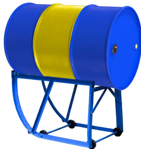
Figure 5. A fuel drum stored horizontally with the vent and bung at the 3 o’clock and 9 o’clock positions, respectively (Source: TSB).
