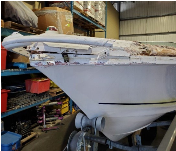
Figure 8. Damage to the pleasure craft's bow and port side (Source: TSB)
