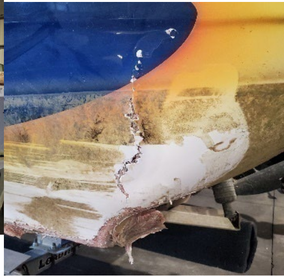
Figure 9. Damage to the pleasure craft's stern (Source: TSB)
