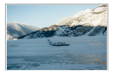
unnoticed by the pilot, and struck the ice. Turn performance calculations indicate that, at 160 knots, the pilot would have to maintain an angle of bank of about 40 degrees (steep turn) to complete a 180-degree turn within the confined valley. The loss of altitude and eventual contact with the ice are results consistent with similar accidents investigated by the TSB.<sup>3</sup>
