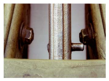
Indications of interaction between the trigger/safety pins and the fitting sub-assembly fasteners were also observed on a comparison aircraft, as shown by damage to the ends of the pins, grooves in the innermost end of the nuts, and thread imprints in the trigger/safety pins (Figure 2).
