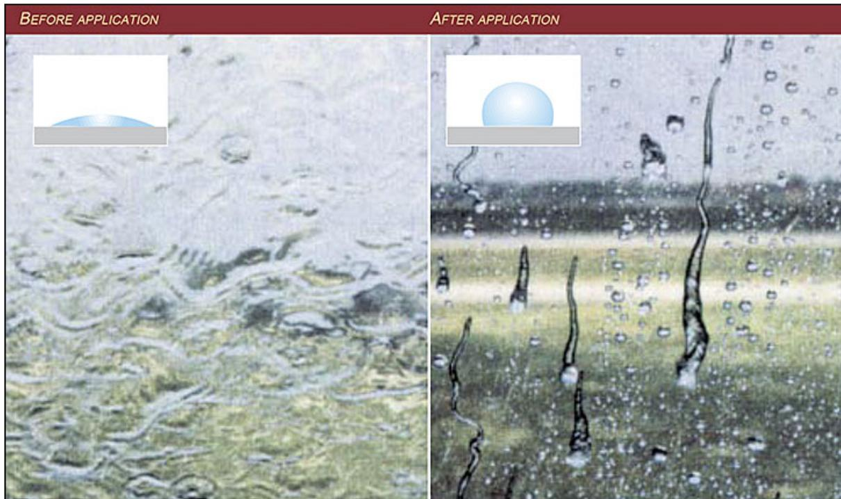
The rain repellent acts quickly and for an extended period without leaving residue or creating distortion, and restores visibility within a few seconds. The surface tension of the windshield, which is temporarily altered, coupled with airflow, prevents drops of water from adhering to the windshield (Figure 3).
