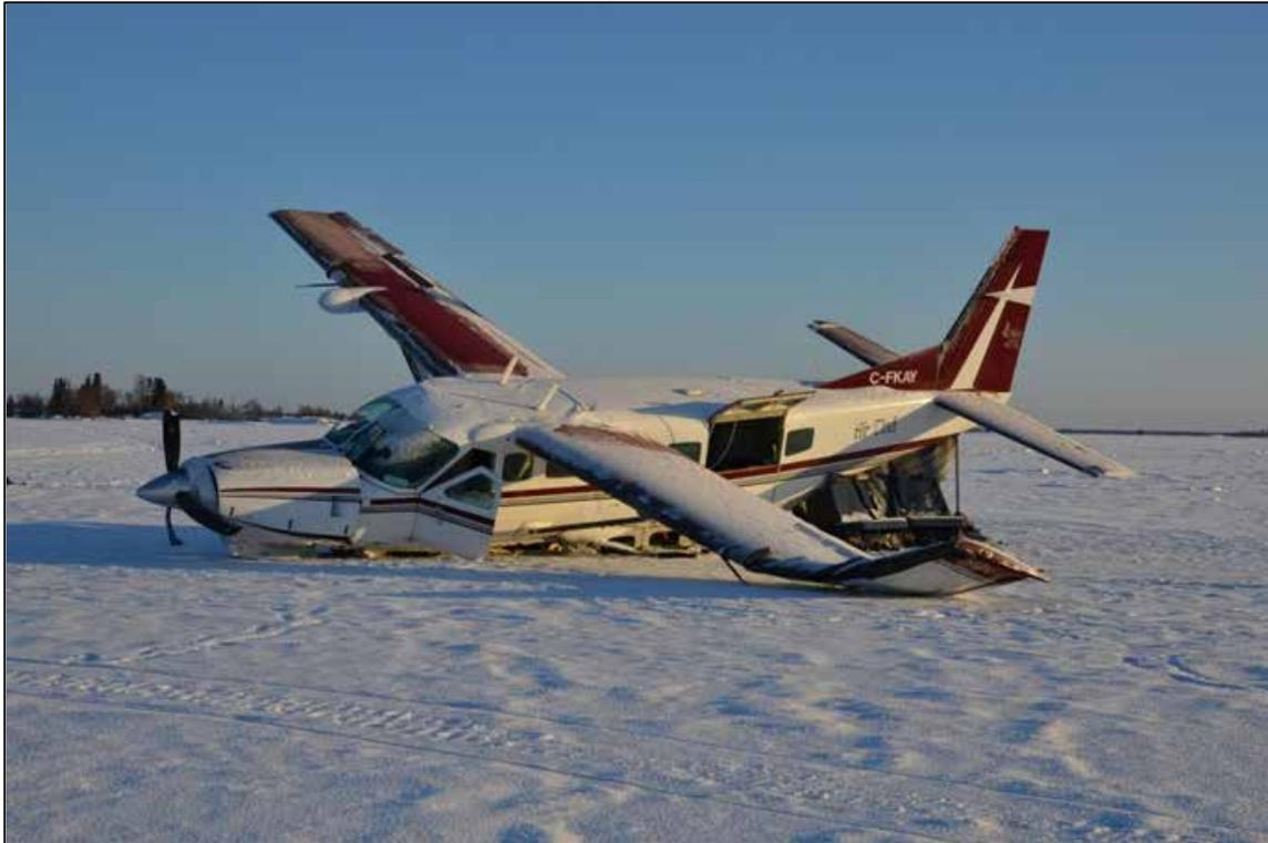
Mixed ice<sup>23</sup> up to 1.5 inches thick was observed on the unprotected surfaces of the aircraft (Photo 2 and Photo 3). Protected surfaces had residual ice. Ice was also observed aft of the protected surfaces, on the undersides of the wings. The windshields were obscured with ice accretion, except for a small area protected by the electrically heated windshield anti-ice panel. The propeller spinner and radome had mixed ice, extending aft to approximately the midpoint of the components.
