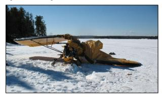
An inspection of all flight control cables did not reveal any pre-impact anomalies. Damage to the engine and propeller suggests that the propeller was rotating and that the engine was producing substantial power at the time of impact.
