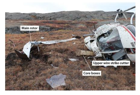
Figure 1. Photo of the wreckage showing the helicopter on its right side, the main rotor and the core boxes (Source: Royal Canadian Mounted Police)
