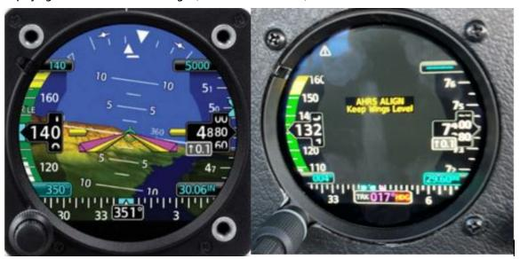
At the same time, the aircraft's horizontal situation indicator (HSI)<sup>4</sup> also indicated a failure, displaying a red X over the HDG (heading) annunciation. The pilot attempted to switch the HSI to the ADI page using the instrument's touch screen function and selector knob, but was unsuccessful.
