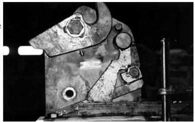
such that it can only open into the hook (see Figure 6). This design feature allows the suspension ring to be inserted into the hook assembly and prevents the ring from inadvertently slipping out. The retaining latch is not designed to carry any significant amount of weight.
