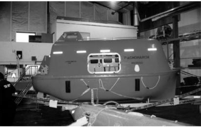
Each lifeboat is powered by an inboard diesel engine that drives a fixed-pitch propeller. Steering is by means of a controllable Kort nozzle.
