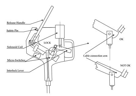
In case the lowering mechanism malfunctions, which could cause the lifeboat to become suspended from the
