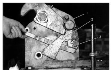
On each hook assembly, the hook, the blocking lever, and the reset lever carry reference marks. The cheek plates have corresponding reference marks. The hook has been correctly reset when these marks are properly aligned.
