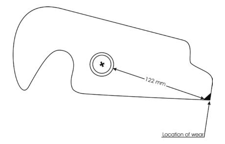
The load-transmitting contact surface on the hook wears with use, reducing the length from the end of its load-transmitting surface to the circumference of its pivot. According to the manufacturer, this minimum distance is 122.0 mm. A shorter length can lead to two effects, both potentially detrimental:
