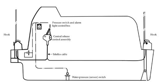
The central release control assembly is just behind and to port of the coxswain's seat (see Photograph 12). It is made of two galvanized steel side plates to which are connected the release lever, the cable connection arms, and the interlock lever. A solenoid coil is mounted on top of the framework formed by the side plates.
