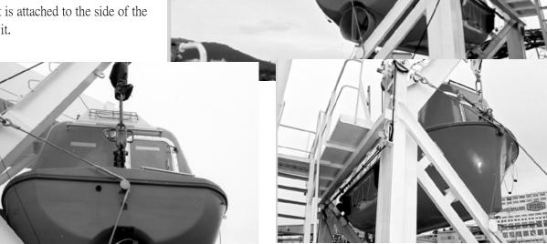
In the lifeboat's stowed position, the free end of this rotating lever bears against the rigid support frame of the
