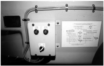
The green lamp also indicates two operating conditions: one when the lifeboat is in the water and it is safe to pull the release handle; the other when the hooks have been correctly reset to the load-bearing position.
