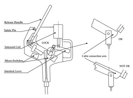
The two cable connection arms are connected to reset levers on the forward and after hook assemblies via teleflex cables in such a way that they form an inflexible structure. When the cable connection arms move upward, under the action of the release handle, the reset levers are forced to move downward.
