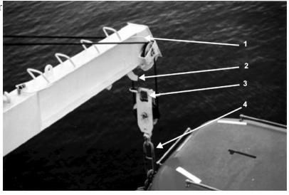
The electric winch has a unidirectional freewheeling clutch and a brake that is activated by a weighted dead man's handle. This handle is also connected to the winch-brake remote-release cable (see Figure 2, Item 9), which passes through another set of sheaves and into the conning tower of the lifeboat, ending within easy reach of the coxswain.
