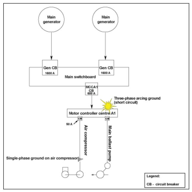
Figure 2. Circuit breaker line diagram
