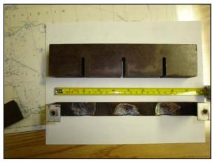
**Photo 13.** View of steel bracket showing result of arcing and bakelite insulation block
