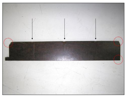
**Photo 9.** View of the 6 mm "H"-shaped bakelite insulation piece as found on the switchboard deck. Arrows show indentations in way of bus bars. Circles show missing tabs.
