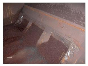
**Photo 6.** Port bilge well, with strainer plates sealed off
