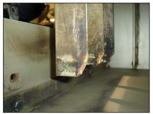
**Photo 12.** End view of bus bars showing result of arcing
