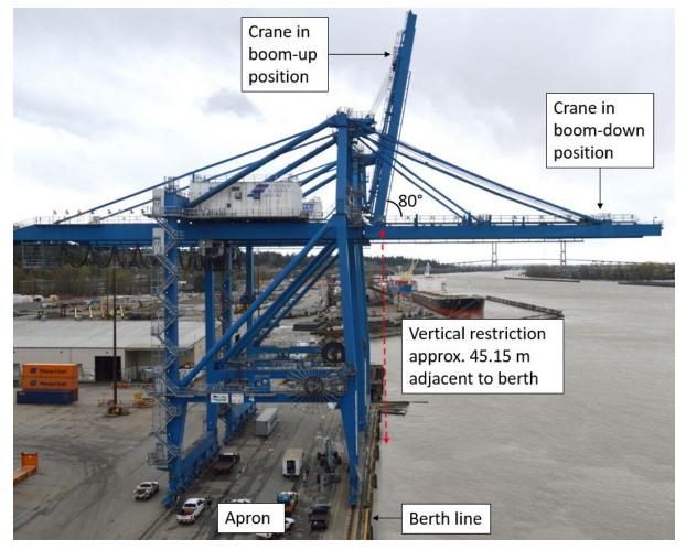
Figure 6. Gantry crane vertical restriction adjacent to berth (Source: TSB)
