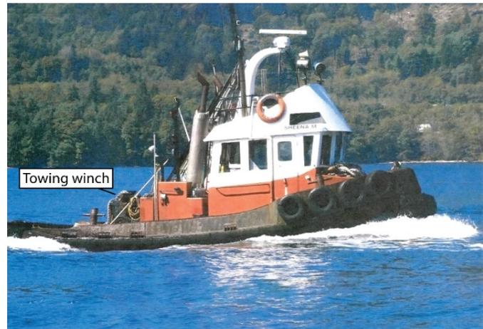
Mills in Port Mellon, BC. At approximately 1230 Pacific Daylight Time, as was his regular practice, the master on the *Sheena M* used a towline without a towing bridle to secure the towline from the towing winch to the barge's port forward bollard.
