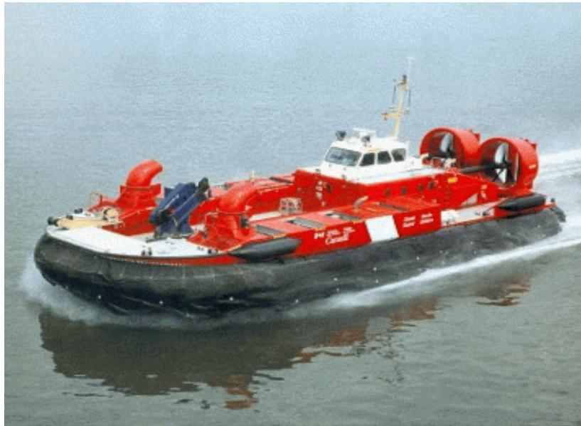
The control cabin of the “SIYAY”, similar in design to that of an aircraft, is near the after end of the craft (see Figure 1). The design allows for an excellent view forward, with the exception of the bow thruster vents to port and starboard at the forward end of the craft, which cause blind sectors. Operationally these blind sectors are overcome by the craft captain and port seat occupant exchanging information as targets move from one sector to the other.
