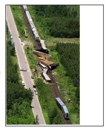
The rails, crossties and roadbed at Mile 1.78 were substantially displaced both longitudinally and laterally. Wheel flange marks on the web of the rail indicated that the rail had rolled over and that loss of track gauge had occurred.
