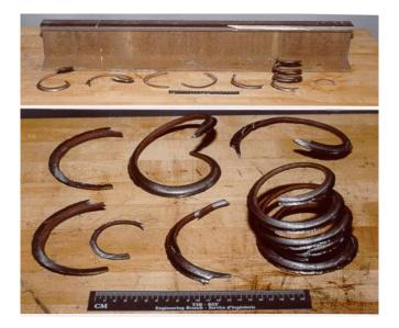
The TSB Engineering Laboratory examination (Report No. LP 71/01) showed that there was a flow lip up to 12 mm thick on the gauge side of the railhead. There was no flow lip on the field side of the rail.
