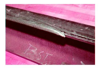
This section of rail consisted of 132-pound continuous welded rail, manufactured by Algoma Steel in 1971. The rails were transposed<sup>2</sup> in 1999, however their installation date is unknown. The sum of the vertical and lateral wear was 27 mm (1 1/16 inches), thus exceeded the 22 mm (7/8 inch) limit specified in Canadian National's (CN's) *Standard Practice Circular* (SPC) 3200.
