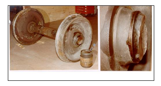
A section of a broken axle journal, with its roller bearing (see Figure 2), was found in the ditch on the south side of the track, at Mile 16.25; it originated from car CNWX 107921, the second derailed car. The car in question was a covered hopper car made of aluminum, with a light weight of 41 000 lb (20 045 kg) and maximum loaded weight of 220 000 lb (100 000 kg). The car's shipping record indicated that it was at its maximum load weight at the time of the derailment.
