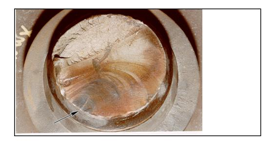
The axle was manufactured by Standard Steel Castings in March 1964, and was reshaped by GE Railcar in 1991. CN maintenance records indicate that new wheels, with 6 inch x 11 inch AP roller bearings, were installed on the axle in February 1994 at the Transcona shop in Winnipeg. The axle was installed at the "A" end of the car (fourth axle from "B" end) on 28 March 1994. All work was performed in compliance with AAR standards.
