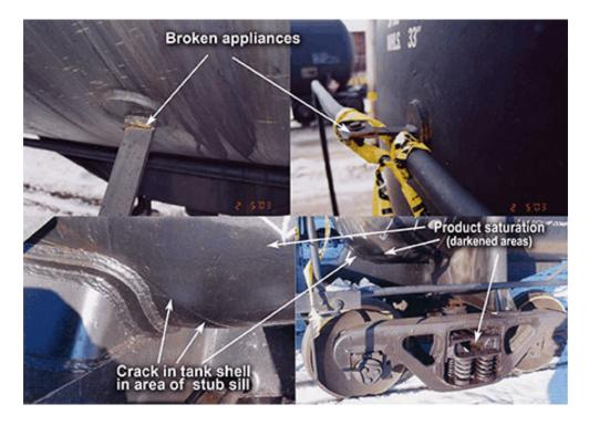
A portion of the tank shell, which included the crack, was cut from the tank car and sent to the Transportation Safety Board of Canada (TSB) Engineering Laboratory for analysis. The examination (report LP 048/2003) determined that there was a pre-existing crack in the tank shell that had been present for a considerable length of time, likely initiated during welding. During the service life of the tank car, it had been subjected to normal service loads without previously failing.
