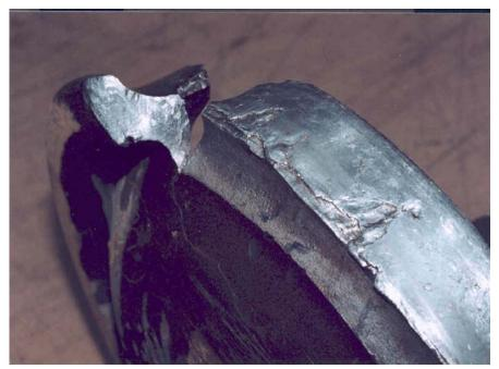
Photo 2. Shelling on the running surface
