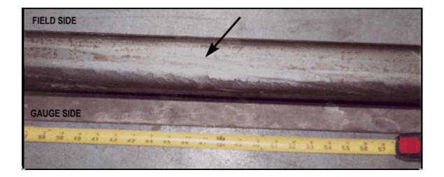
There was no evidence of polishing or of batter marks on the rail fracture surfaces, or on the fracture surfaces of the broken joint bars. However, one joint bar on the west rail and a second joint bar on the east rail exhibited some pre-existing fatigue cracks.
