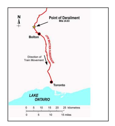
Train movements are governed by the Occupancy Control System/Automatic Block System, authorized by the *Canadian Rail Operating Rules* (CROR), and supervised by a rail traffic controller located in Montréal, Quebec. An average of 16 freight trains per day traverse this area at a maximum permitted speed of 55 mph. No temporary slow orders were in place in this area on the day of the occurrence.
