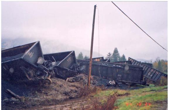
**Photo 1.** Derailed bathtub coal cars from the middle of the consist
