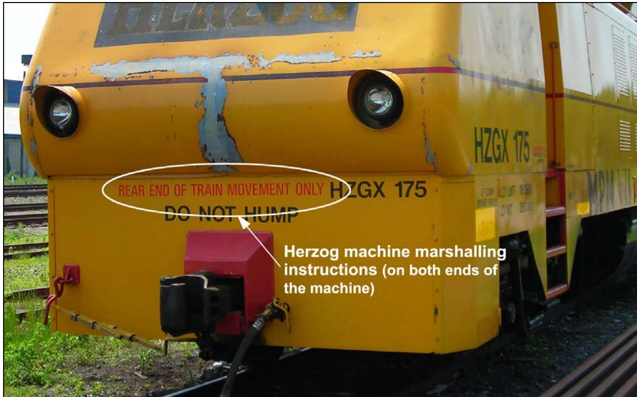
**Photo 8.** Herzog machine (locomotive HZGX175)
