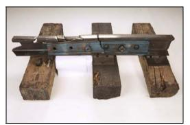
**Photo 2.** Field side view of the reassembled compromise joint (train direction was from right to left)
