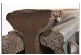
**Photo 3.** Fatigue crack at the upper inboard corner of the joint bars
