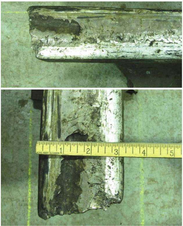
**Photos 2 and 3.** Fracture at the south end of the 3 mating west rail pieces showing material flow and heavy checking on the gauge corner. A 10 inch long section of rail head was crushed measuring approximately 7/16 inches at it deepest point. Corresponding shelling was also observed on the running surface at the fractured south end.
