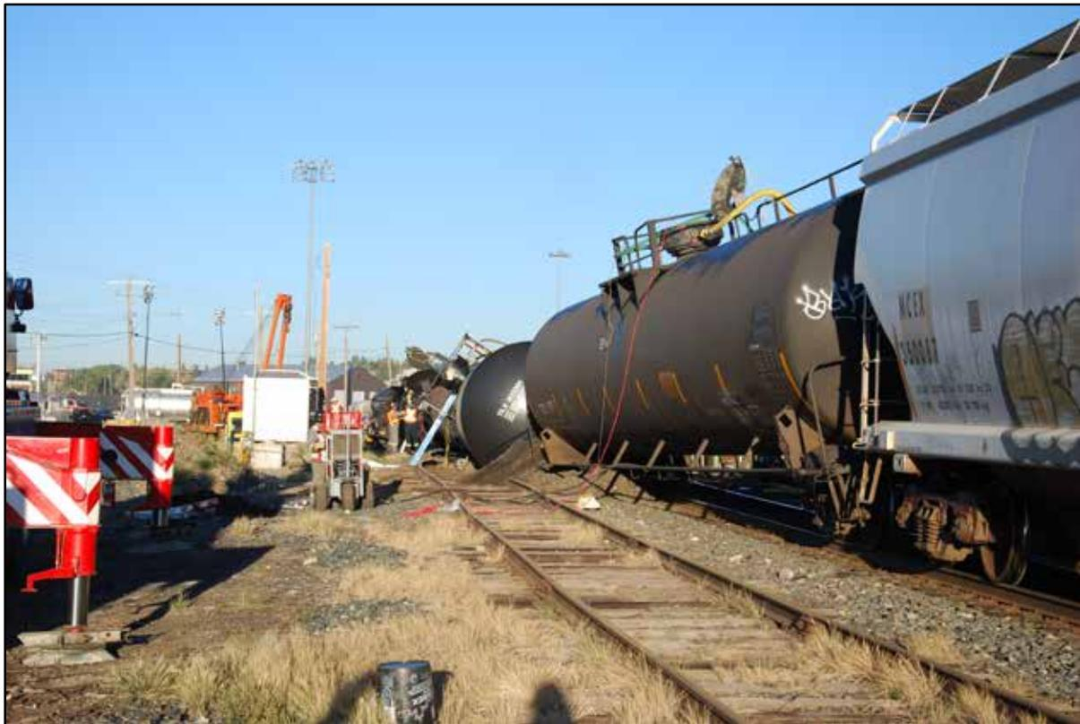
The derailed tank cars were loaded with liquid hydrocarbons, not otherwise specified (N.O.S). The product was placarded as UN 3295, which is commonly referred to as natural gasoline condensate or natural gasoline (see Photo 2). This product is most commonly used as a diluent for bitumen<sup>4</sup> to lower its viscosity so it can flow through pipelines.
