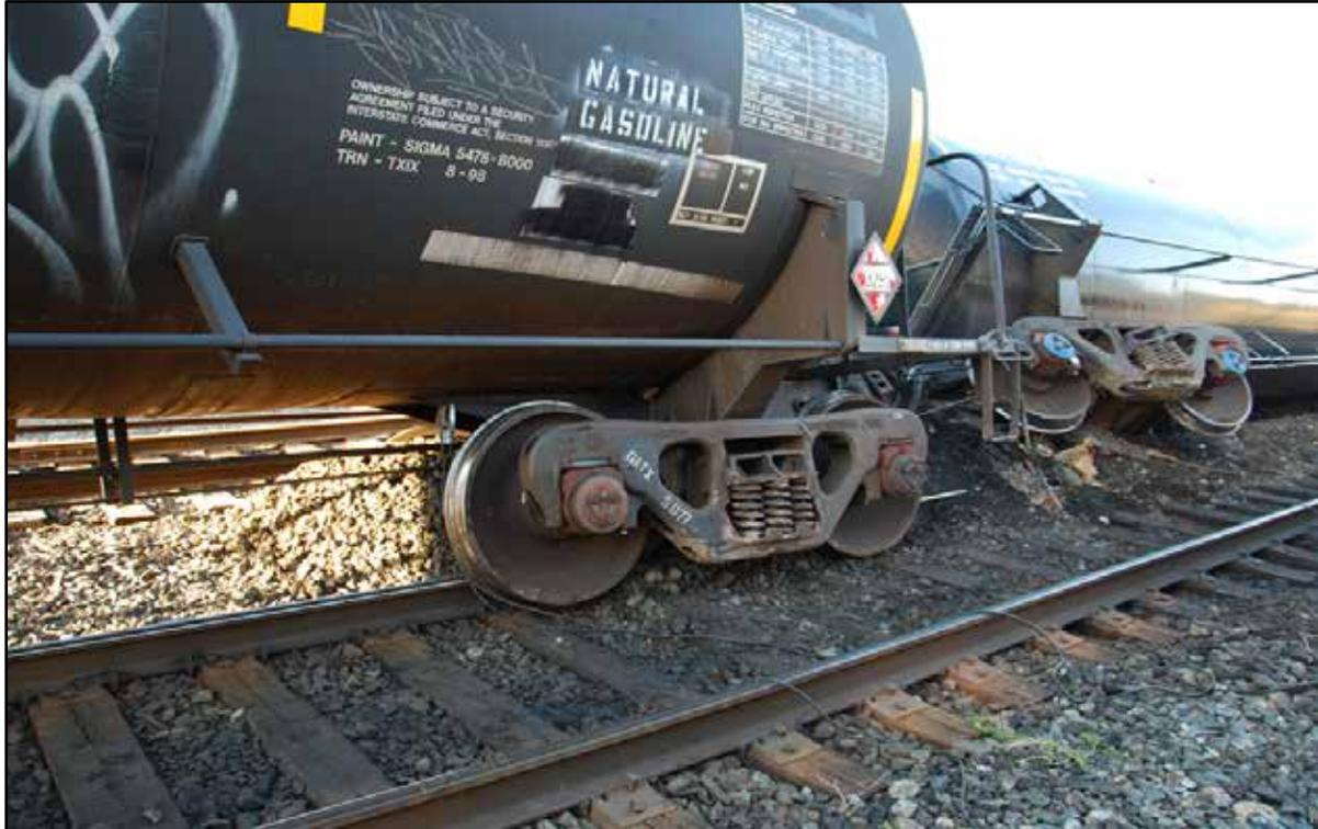
The point of derailment was determined to be at Mile 0.3, where there is a crossover from the Alyth Yard track to the Red Deer Subdivision. Impact marks and flange markings were observed post-accident on the running surface of the right-hand switch point of the divergent route of the turnout (see Photo 3). Wheels had climbed up on top of the switch point and had travelled along the top of the rail before falling between the point and the stock rail.
