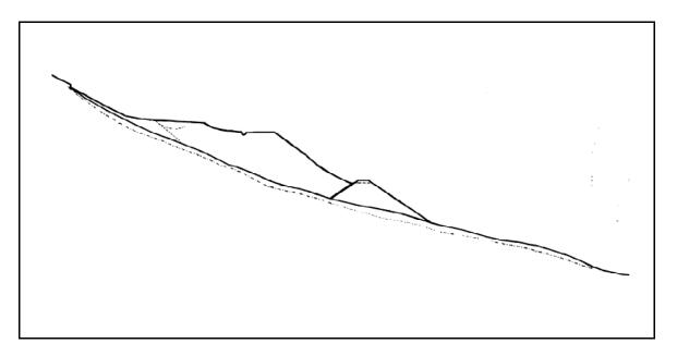
The railway subgrade was built in 1915 using local fill materials laid on *in situ* ground material. In 1979, the railway built a parallel siding track west of the main track. The additional fill for the siding embankment, composed of granular material, was also placed on the original ground surface material.
