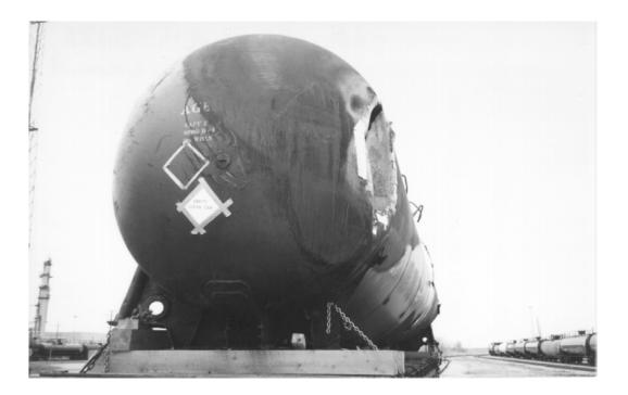
The tank car of LPG, CGTX 63501, was built to specification DOT-112J340W. The tank car was heavily damaged but experienced no loss of product.
