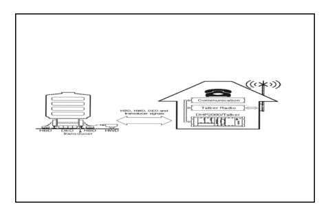
Today, HBDs are strategically placed throughout the core network of most major railways. The principal target of the detectors is freight car bearings (which comprise about 97 per cent of all axles). CN has 68 subdivisions protected by HBDs, representing over 97.9 per cent of CN's traffic. Of the remaining 48 subdivisions, 11 are under 20 miles in length and account for
